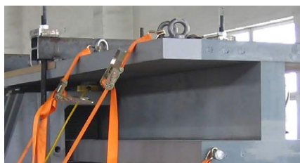
Preparing the special bearings for transport
