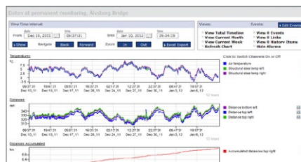
Presentation of measured data (in graphic form) from the applied SHM system
