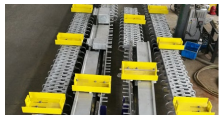
TENSA®FINGER RSFD finger joint during production in the factory
