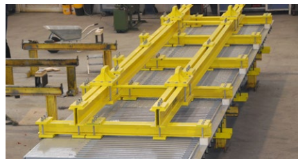
Sliding finger joint with transportation and installation frame, ready for delivery
